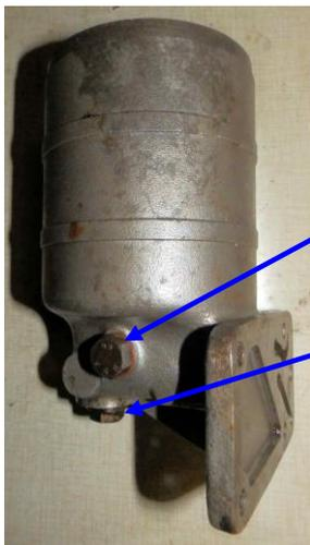
There is the 30mm long screw at the side of the bowl. Unscrewing this screw about 12 – 15mm will drain most of the oil in the bowl to down below the level of the filter itself. To get rid of the remaining oil, about 8mm or so, left in the bowl, there is a drain plug in the centre of the base. I suppose you would only undo this plug if you really wanted to clean out the bowl and any sludge which may have collected there.
